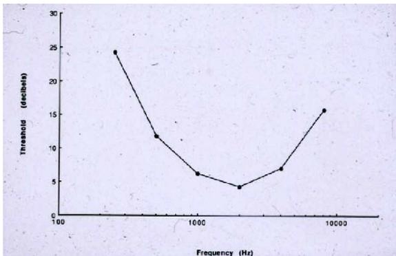
Each point of the curve is a normative threshold level at the selected test frequency; all curve points possess a corresponding sound pressure level (SPL). By definition, each point of the threshold curve becomes 0 dB HL. It is important to note that 0 dB HL does not refer to absence of sound; 0 dB HL corresponds to a measured normative sound pressure level in humans at a particular test frequency.
